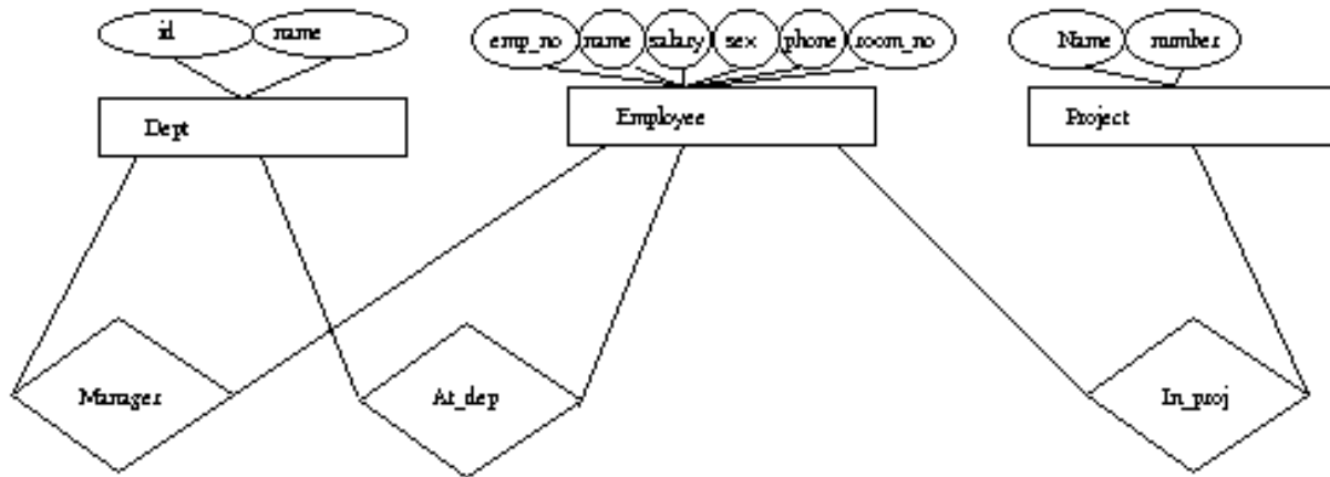
Figure 3.1: Company Entity-Relation Diagram
